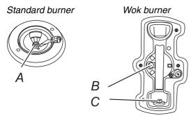
A orifice, B internal injector, C external injector Remove burner caps and heads. Remove old orifices, save the orifices removed from the appliance for future use. Fit new orifices. Reassemble in reverse order.
